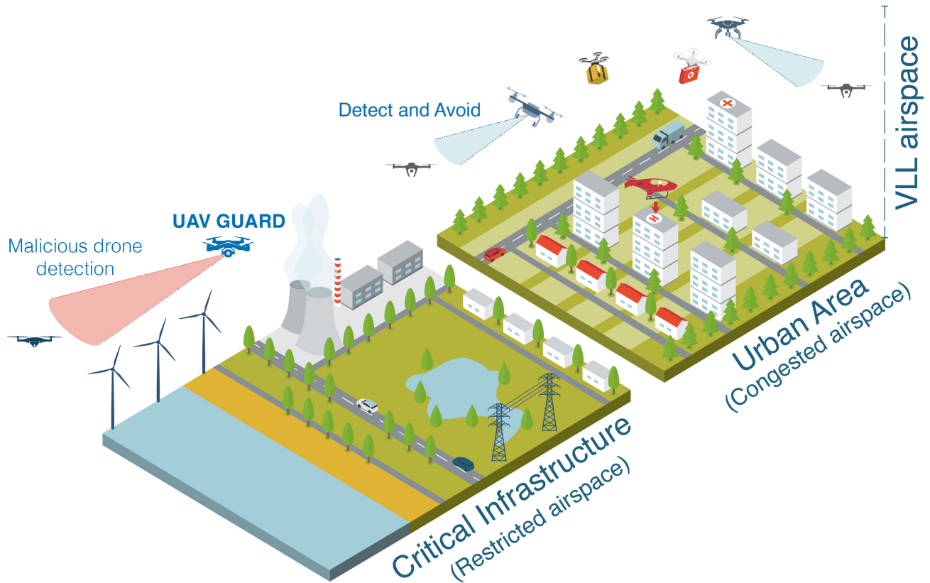
Fig. 1. Illustration of UAS-borne radars monitoring restricted airspace and supporting the safe operation of drones in congested airspace.
